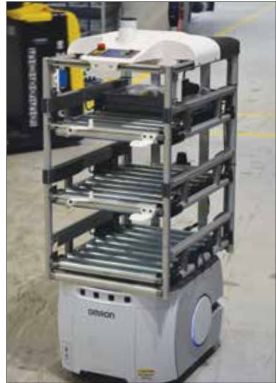
OMRON robot used by Lectra in its factory for material movement
