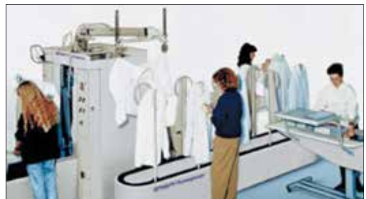
Veit- Kannegiesser H-PV2, for pressing the entire body of the shirt in one operation. It is equipped with an automatic unloader.
